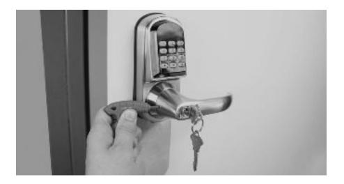
Remove the handle and turn it to the left. The handle will be correctly mounted if the bolts are not pressed inward.
